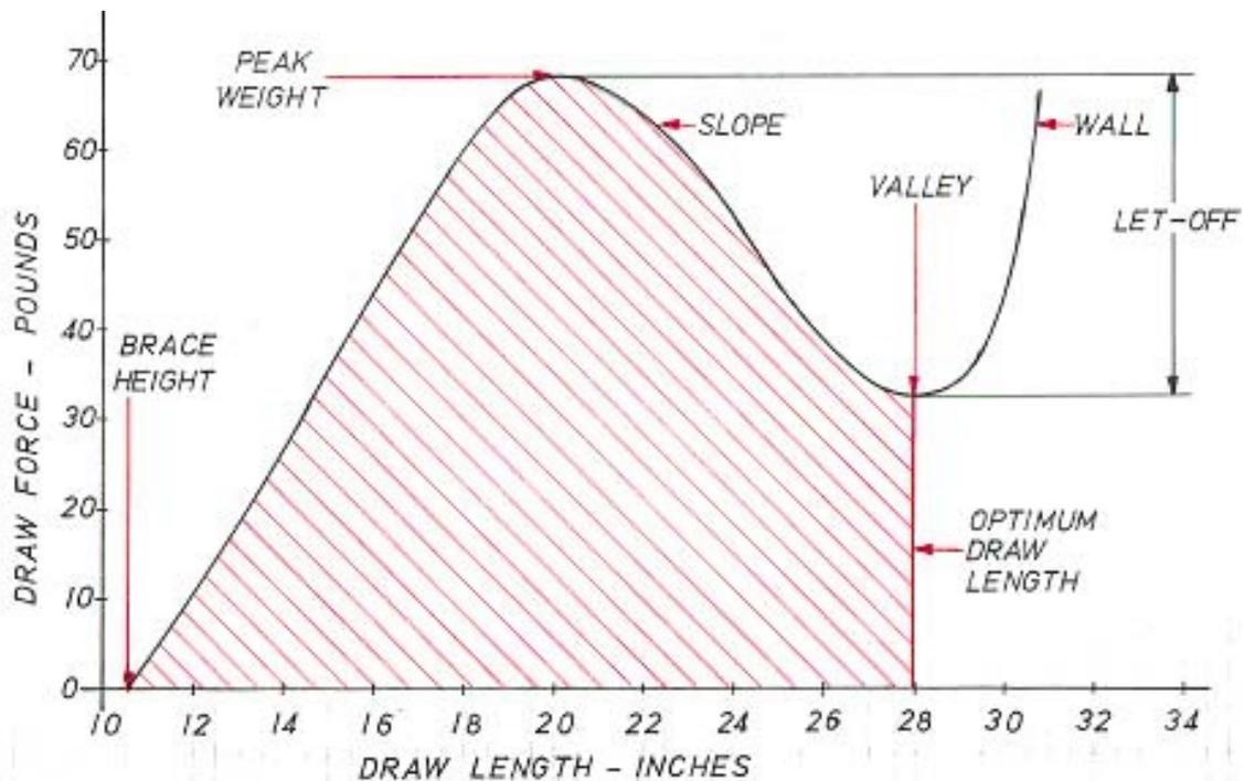
By plotting the Draw Weight up the vertical axis and Draw Length along the horizontal axis shows how the force increases as the bow is drawn, reaches a peak, then reduces as we approach the valley. The area under the curve can be calculated and shows the amount of energy stored by the bow.
