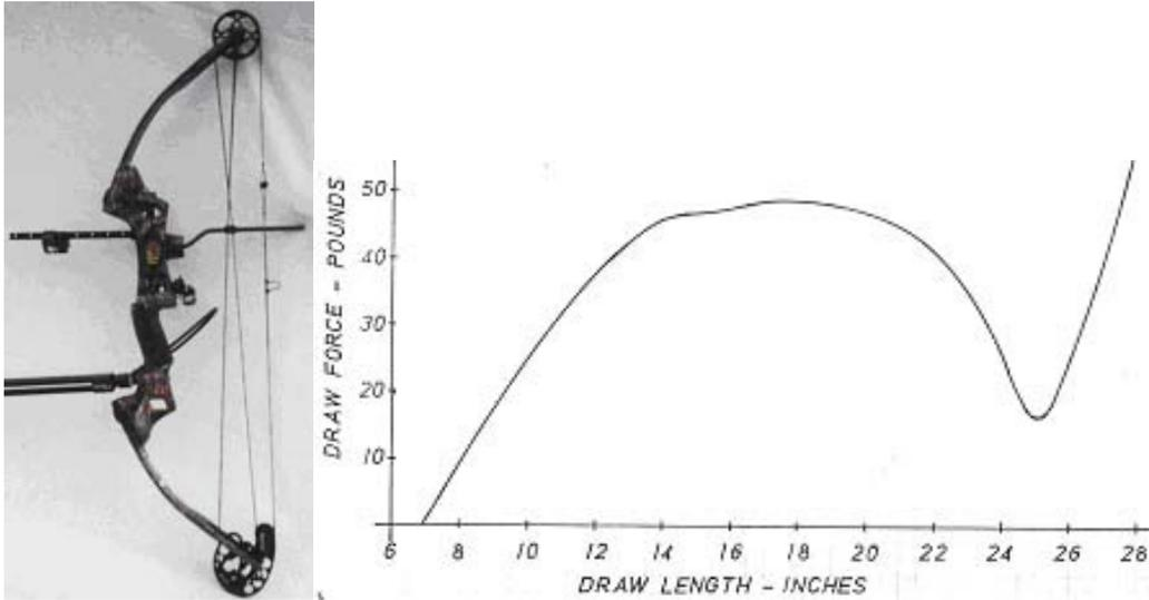
Above is an example of a short bow, 32ins Axle to Axle, with a single cam together with its Force Draw plot. As you can see this is much fuller and therefore stores more energy than the longer target bow with mild cams. Notice also that the “Valley” is now shorter and more clearly defined, improving shooting consistency.
