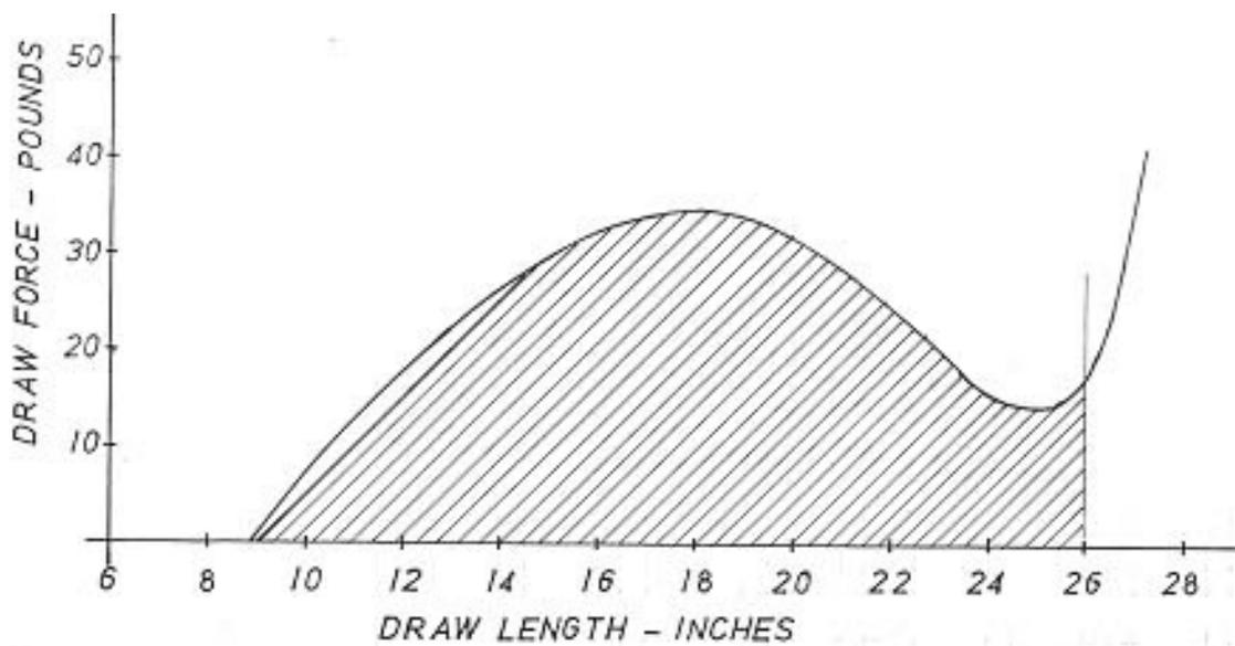
If the two Force Draw plots are put together, it is easy to see that the Compound bow stores much more energy than the Recurve. This explains why the arrow will be launched with a much higher acceleration and ultimate speed.
