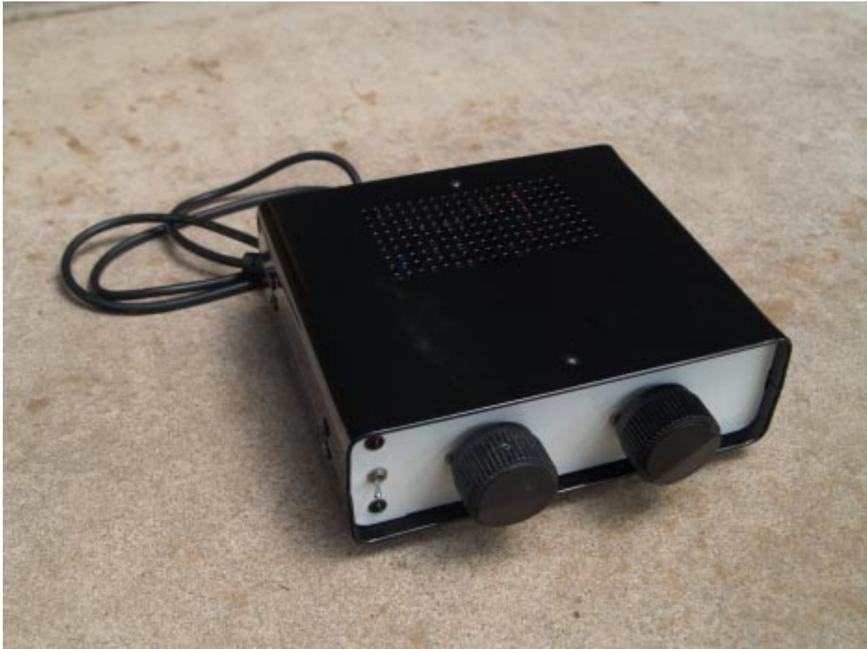
Antenna Interference Canceller (Front View)
