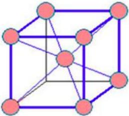
This mineral is an alloy of iron and nickel which is found on Earth only in meteorites. Kamacite has 5-10 wt% Ni, and in the cubic system is body centered cubic (BCC). In the image the center atom within the cube can be seen.
