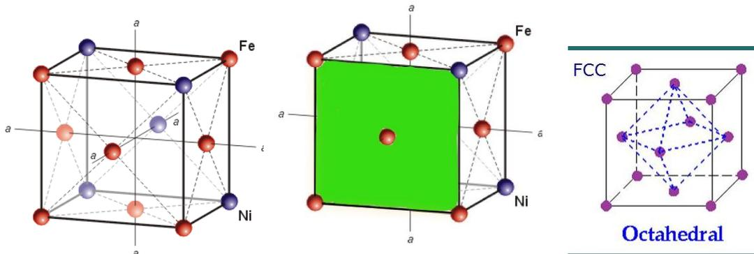
The middle diagram shows one face of the crystal to show the FCC type. Inside there is an 8 sided set of crystal planes. These form an octahedron from the atoms on the faces. An FCC structure has close packed octahedral planes. These minimum atomic spacing planes are the faces that allow Kamacite to grow into Taenite to create the Widmanstätten/Thomson structure. FCC crystals can be thought of as stacked octahedral planes.
