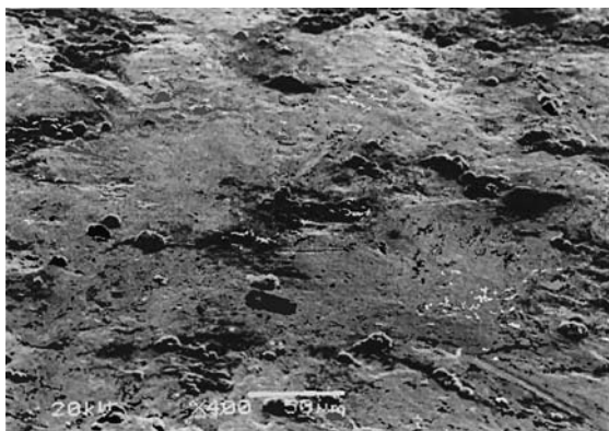
Fig. 9.17 Scanning electron microscopy image: preexisting deposits on the surface of a brand-new and unfired 9-mm FMJ bullet. Most contaminations presented in the form of small spherical Al-Si-combinations
