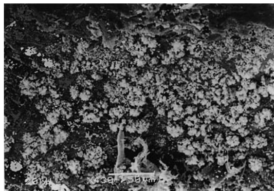
Fig. 9.19 Scanning electron microscopy image: gypsum-board deposits on a 9-mm FMJ bullet after perforation of gypsum-board
