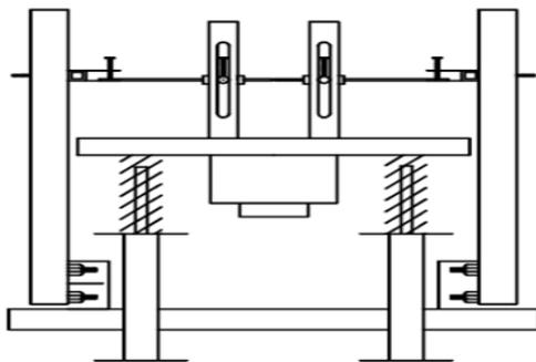
**Fig.1:**Supporting device for welding.
