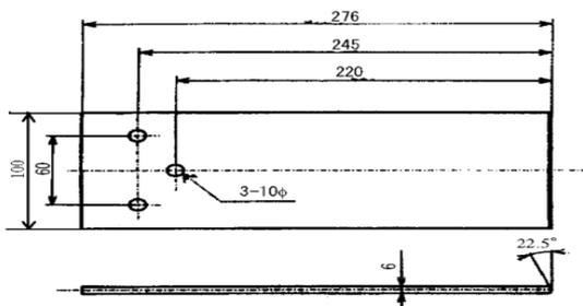
**Fig.2:** Size and shape of specimen made of EN8 steel for general structure
