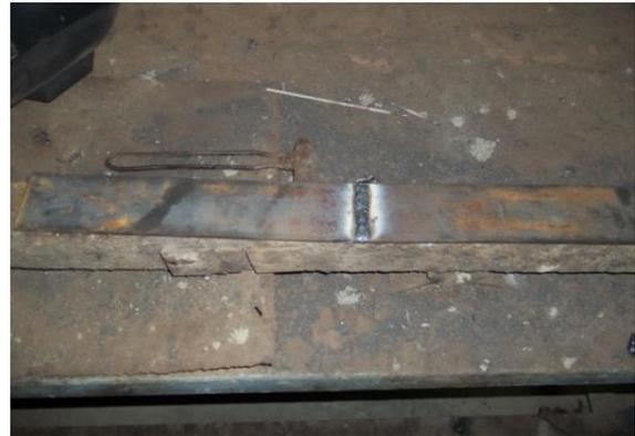
**Fig 4:** welded specimen plates with vibration load
