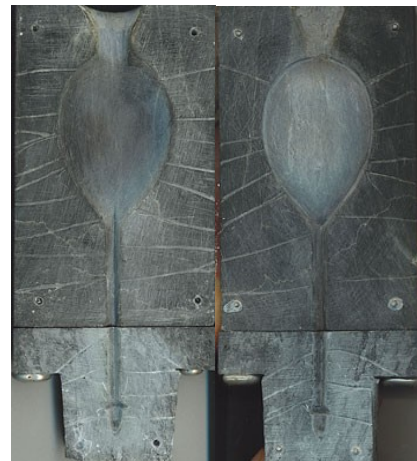
Figure 9. My mould, female and male respectively
